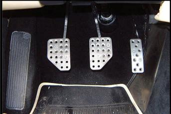
The 355 well measures just over 13" from the side of the white kick plate on the right across to the side of the dead pedal on the left, measuring across the bottom of the brake and clutch pedals. The 550 well measures just under 14" across the bottom of the pedals. I have not tried to tweak the pedal positions on the 355. Note that the 550 offers more configurability than the 355 for the brake and clutch pedals.
